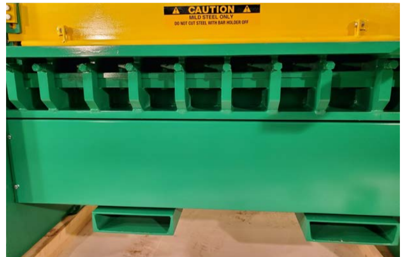
BLADE GAP MICRO ADJUSTMENTS ALL DOWN THE BLADE
